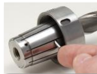
Insert Pin into the Pin Hole Note: if cutting tool flat is not in the correct orientation the pin will not insert, rotate cutter if needed to align the pin to the flat
