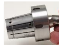
Once the pin is fully inserted pull out on the cutting tool so the back of the flat is tight against the pin
