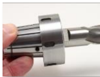
Insert cutting tool into the collet, cutter flat orientation to the pin hole as shown
