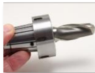
Fully insert cutter into the collet
