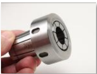
Insert SX25-NP Collet into the SXN25M Nut
