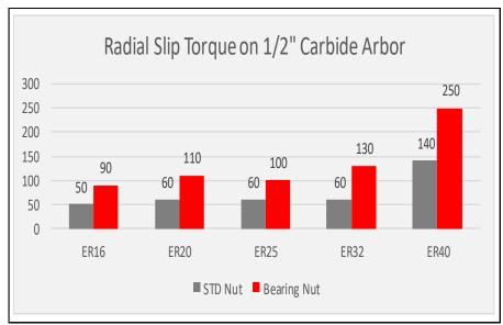
ER32 standard nut locked at 100 ft/lbs using a 1/2" carbide test arbor, the arbor slips at 60 ft/lbs of radial torque, using a Pioneer Bearing Nut the arbor slipped at 130 ft/lbs of radial toque. The average improvement on ER16 thru ER40 was 75% to 125% increase in radial holding power.
