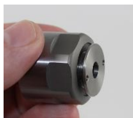
Thread Coolant Cap into ER nut, snug with wrench after the collet has been assembled.
