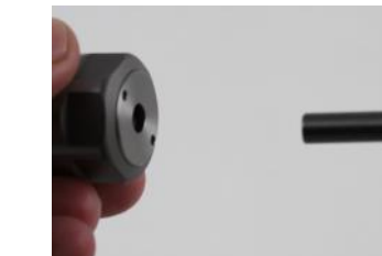
Insert cutting tool with the seal engaged on the round part of the shank
