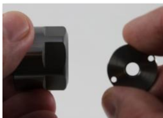
Thread Coolant Cap into SX nut, do not tighten, assemble the collet.
