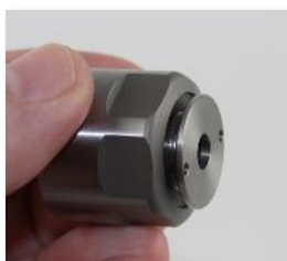
Thread Coolant Cap into SX nut, do not tighten, assemble the collet.
