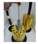
Note: If the cutting tool has broke in a way to damage the bore of the Shrink Fit holder, this procedure will not work, the tool will not push out.
