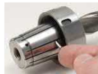
Insert Pin into the Pin Hole Note: if cutting tool flat is not in the correct orientation the pin will not insert, rotate cutter if needed to align the pin to the flat
