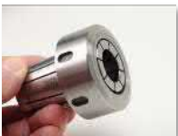
Insert SX25-NP Collet into the SXN25M Nut
