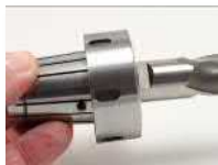
Insert cutting tool into the collet, cutter flat orientation to the pin hole as shown
