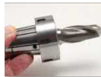
Fully insert cutter into the collet
