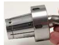
Once the pin is fully inserted pull out on the cutting tool so the back of the flat is tight against the pin Use safety gloves if required
