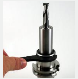
Tighten locking collar to 30 ft/lbs Maximum Do not over tighten or tool can jam or cause excessive TIR!
