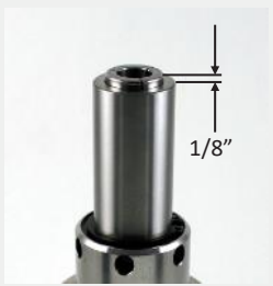
Turn collet until it stops or reaches 1/8" from the face of the chuck. Assemble loose, Do not tighten! Thread gap is required for proper function.
