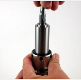
Insert cutter, while holding the cutter hand tighten the locking collar clockwise until the collet holds the tool.
