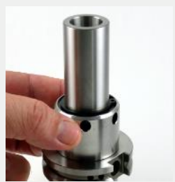
Turn locking collar counter-clockwise until it stops.
