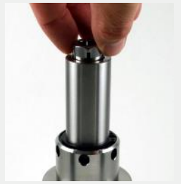
Insert collet and turn clockwise. Use Flat Screw Driver if required.
